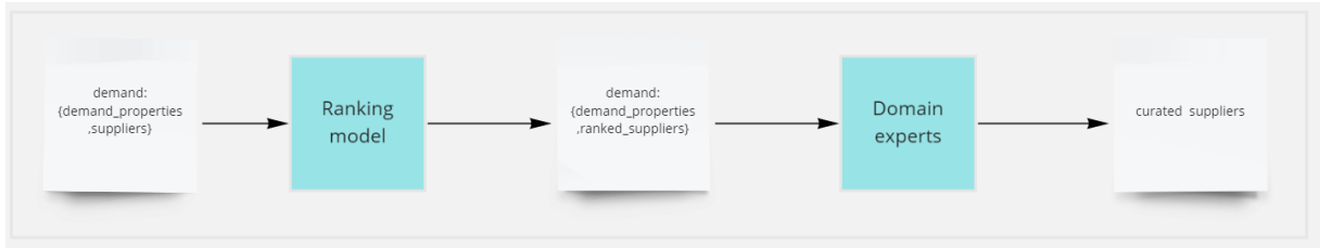
Figure 1.1: Ranking model with human-in-the-loop. The demand consists of demand_properties and an associated list of suppliers, which is consumed by the ranking model. The ranking model sends the ranked suppliers based on the demand to the domain experts, who will then provide the curated supplier list to the customer.
